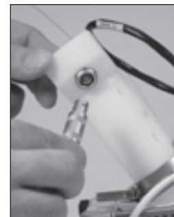
FIGURE 12: Connection of the high-voltage cable to the HV contact on the probe
