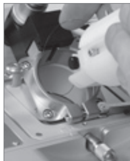
FIGURE 9: Carefully roll excess column length at the front into the probe port
